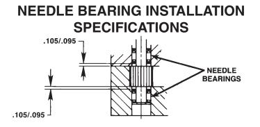
When replacing the needle bearings on the drive gear of the basic pump, the dimensions shown must be as specified.
