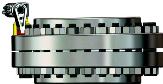
Uneven load using one tool
