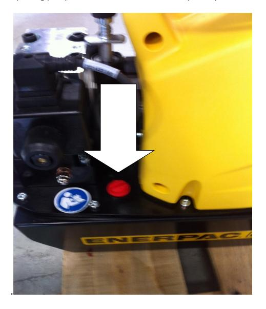
This cap is required when shipping the pump to insure oil does not spill from the reservoir during transport.
